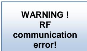
This message will be sent when RF communication is lost between V24 Central and RF antenna of GSM module.
