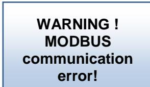
This message will be sent when BUS communication is lost between GSM module and V24 Central appear or with the antenna if Wireless version.
