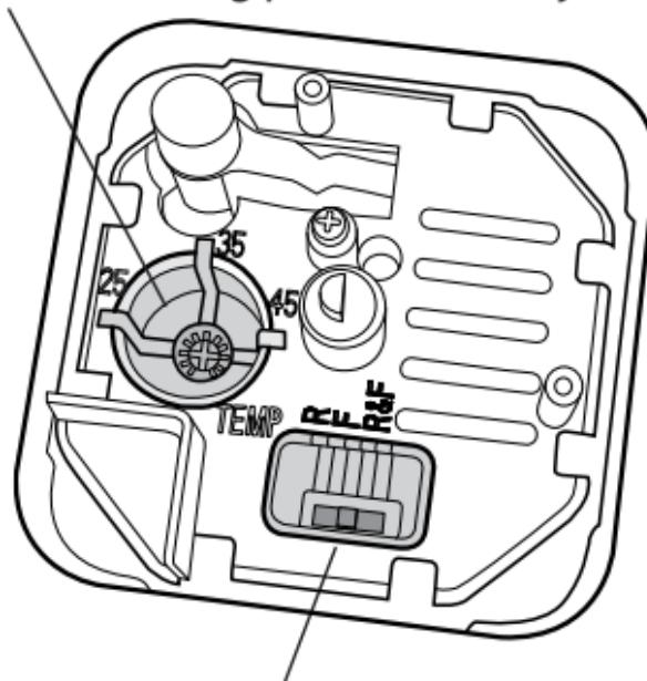
The regulating function is adjusted here.
