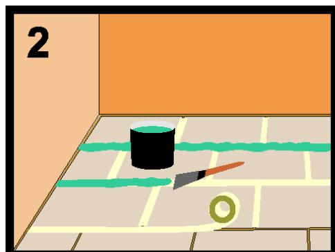
The spaces should be covered with a reinforcing gauze fabric tape. Place the tape, apply the Beta Form H01 adhesive material, spread the residual material with a spreader or remove it. The tape should overlap at least 50 mm. The boards need not be protected with additional hydroinsulation. Allow the adhesive material to harden, as described in the instructions for use.
