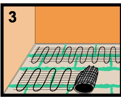
Place the heating mat accordingly for the desired heating area. Apply a layer of flexible sealing cement onto the heating mat and then place the floor tiles. Follow the instructions for their use when laying the heating mats (cables). The expansions joints in the surface finish must not be immediately above the corresponding spaces between the F-boards. The underlying expansion joints must be preserved.
